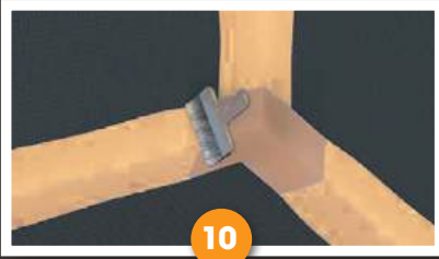
10 Seal all corners of shower area with inside corner membrane / paste.
